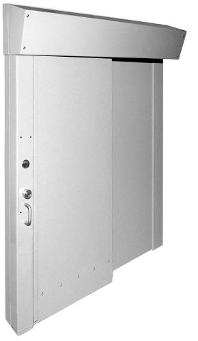
The 7350 is a maximum security, electrically powered, motorized rack and pinion sliding door device for use in applications requiring full remote control of sliding doors. It provides for remote unlocking, locking and movement of sliding doors for entrances, safety vestibules and corridors. The drive system provides precise control and smooth operation.
