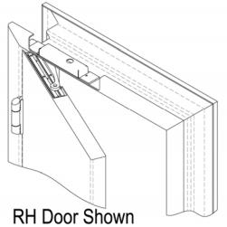
A MORTISED MECHANICAL HIGH SECURITY DOOR POSITION SWITCH
