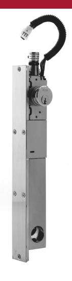
The **9500** provides for pneumatic or manual locking / unlocking of swinging and sliding doors with vertical engagement of the latch bolt for locking. It can be operated from a remote location or by key at the door. For additional security, it is recommended that the 9500 lock be used with an Airteq high security door position sensor. An automatic door closer may also be used.
