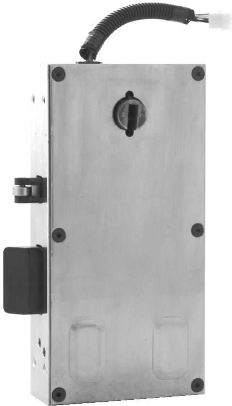
The **9724P** provides for electric or manual locking / unlocking of swinging doors. It can be operated from a remote location or by key at the door. For additional security, it is recommended that the 9724P lock be used with an Airteq high security door position sensor. An automatic door closer may also be used.
