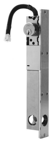
The **9524** provides for electric or manual locking / unlocking of swinging doors and sliding doors with vertical engagement of the latch bolt for locking. It can be operated from a remote location or by key at the door. For additional security, it is recommended that the 9524 lock be used with an Airteq high security door position sensor.
